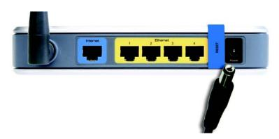
Figure 4-5: Connect the Power
